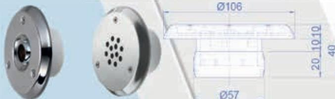
Body made of highly resistant ABS material and face made of stainless steel AISI-316. Available eyeballs: STANDARD or SAFETY (EN-13451 compliant). Designed for concrete swimming pools. Oscillate base allowing up to 12° inlet adjustment. Flow rate:
