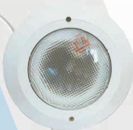
Flat halogen underwater light without niche. Made of white abs plastic. Light screen in transparent polycarbonate. Supplied with 100W/12V bulb and 2.5 m cable.
