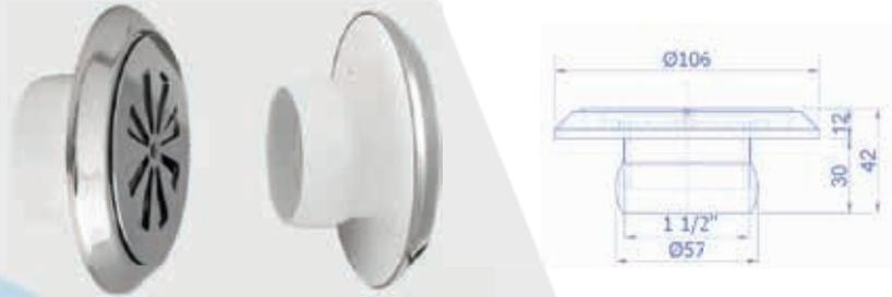
Injection moulded bottom inlets made of ABS or of ABS and stainless steel AISI-316. The top part of this inlet is flat shaped. Adjustable flow rate. Suitable for concrete pools. Oscillate base allowing up to 12° inlet adjustment. Flow rate: 14 m<sup>3</sup>/h..
