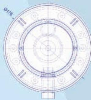
White ABS plastic pool or spa lamp, ideal for constructions with white equipment available in daylight white or RGB colors with a choice through 14 lighting programs while it is equipped with a 30W, or 45W resin led lamp that does not allow water to penetrate inside of. The luminaire with a total diameter of 176 mm and a thickness of 30 mm is provided with a wall socket, 1 m hose and 2.5 m cable. It is an excellent choice for concrete pools and liner pools.
