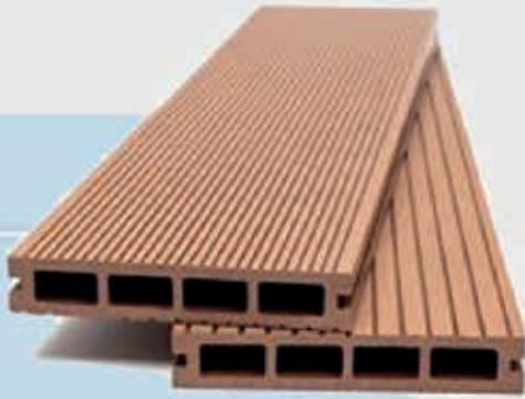
Deck WPC synthetic outdoor flooring composed of 55% wood and 35% HDPE and 10% resins, UV stabilizers etc. It is double sided with narrow comb on one side and wide on the other. Ideal choice for swimming pool floor, terrace, outdoor areas of shops, gardens, marinas, etc.
