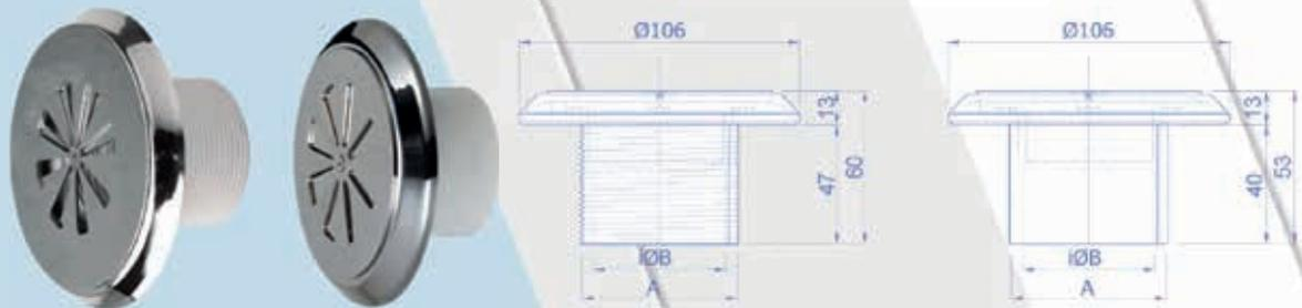
Injection moulded bottom inlets made of ABS or of ABS and stainless steel AISI-316. The top part of this inlet is flat shaped. Adjustable flow rate. Suitable for concrete pools. Flow rate: 14 m<sup>3</sup>/h..
