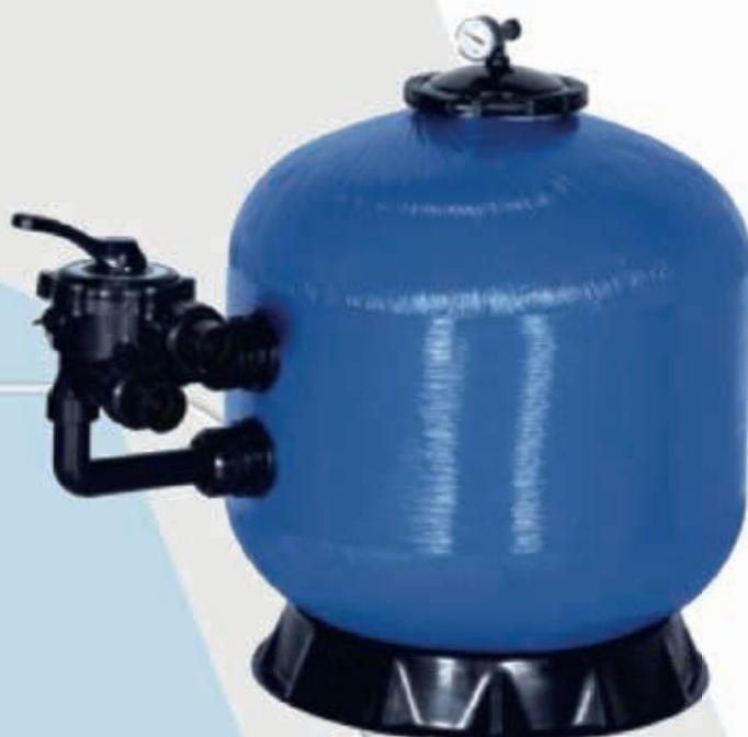
Side mount Bobbin Wound filters are built to be tougher, longer lasting and better performance. Manufactured of polyester resin and non-corrosive-fiberglass filament winding, all internal components and connections are injection molded PVC. Higher filtered water volume with less pump HP. UV-resistance surface allows placement in exterior under sunlight. High quality selection valve is included.
